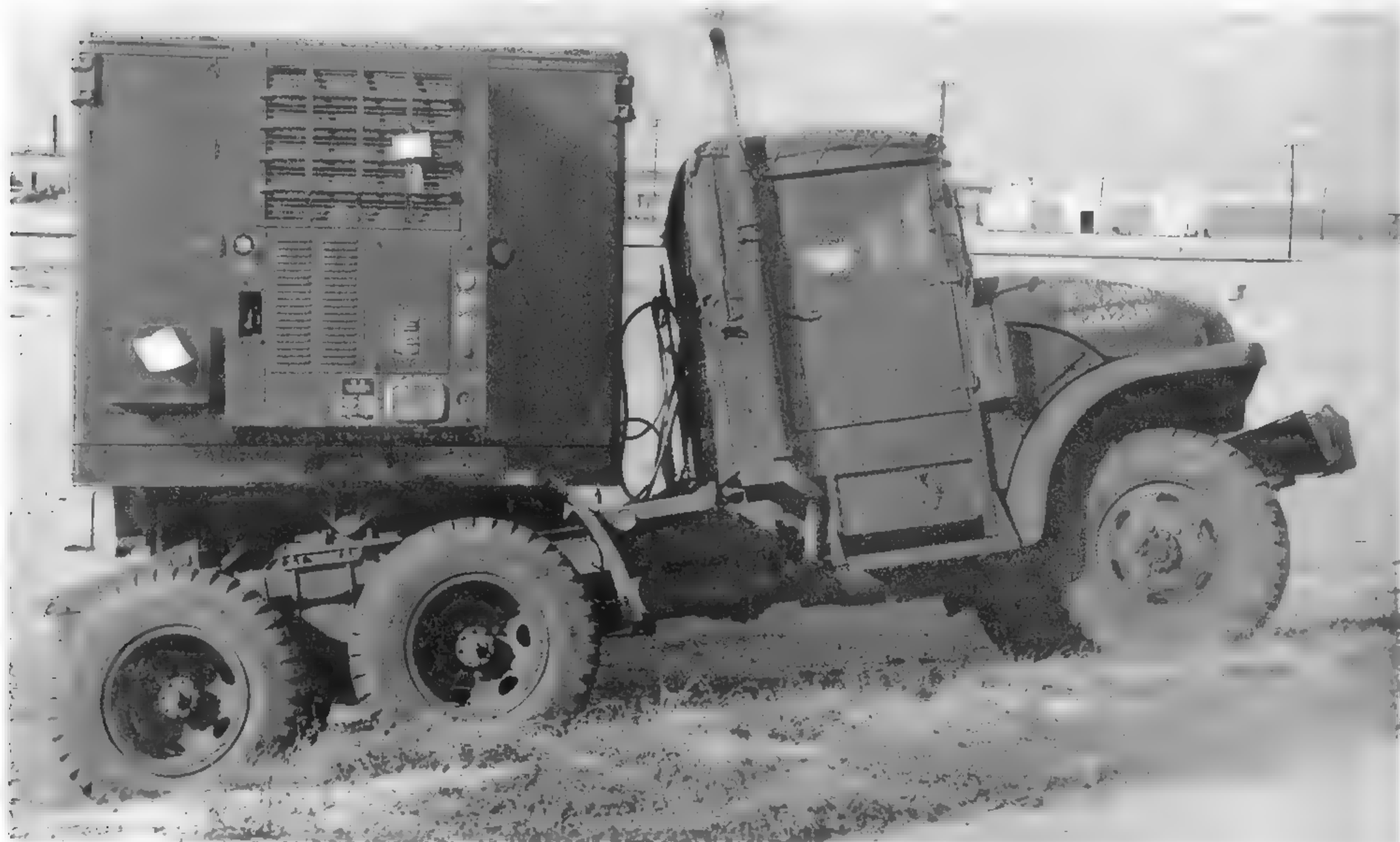
Because of the shorter wheelbase (a benefit in tight turns), the M221 was equipped with a shorter, deeper fuel tank than those used on other cargo trucks. The M221 tractor trucks were not provided with spare tires. The M221 tractor shown here is coupled to a trailer equipped with a Thermo-King refrigeration unit. (Photo courtesy of the Patton Museum)
